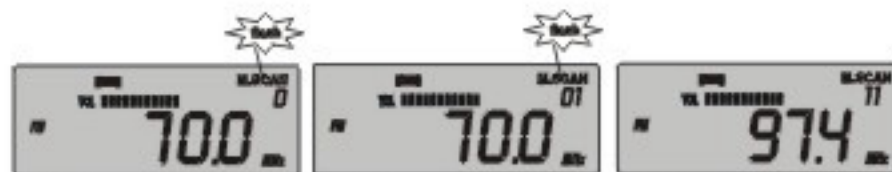
With the memory search state, key in the numeric button "0" / "1" / "1" display progress
