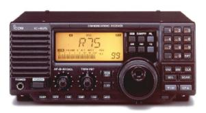
Kiwa Electronics. With those modifications installed this receiver has good audio, a usable sync AM feature, and is at least as sensitive for mediumwave DX as any other receiver I've tried. Surprisingly the receiver has a better frontend than most other well regarded receivers, particularly when considering that the MW attenuation pad has been completely removed. The addition of good crystal filters in the second and third IFs will make this set hard to beat.
